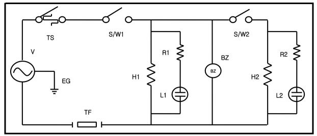
V: Voltage (AC120V, 230V), S/W1: Switch1, S/W2: Switch2, H1: Heater1, H2: Heater2, EG: Earth Ground, R1: Resistor1, R2: Resistor2, L1: Lamp 1, L2: Lamp 2, BZ: Buzzer,
